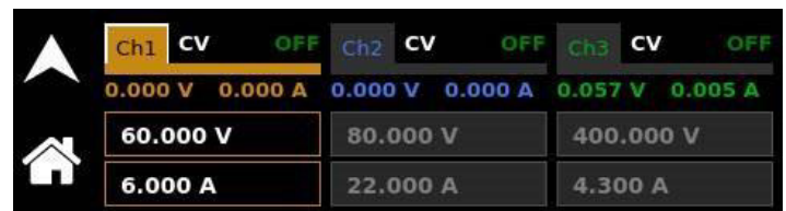
Figure 4. This Dashboard top-level menu shows parameters for each channel with channel 1 highlighted.
