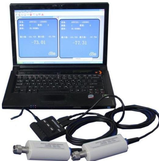
Fig. 3.4 Multi-channel power test with USB HUB
