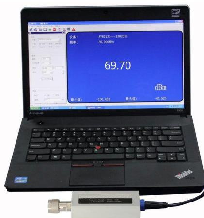
Fig2.2 Connecting the USB CW power senor to the computer
